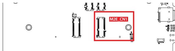
The M.2 key E connector is suitable for applications that use wireless connectivity including Wi-Fi, Bluetooth, NFC or GNSS. Module card types include 2230.
