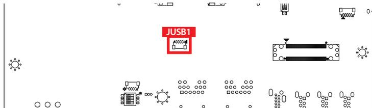
The USB Connector is reserve for GPS function. The USB Bus is switched by software control.
