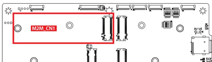
The M.2 key M connector is suitable for applications that use Host I/Fs supported PCIe Gen 4 x4, it can be plugged NvME Module card 2280 type.
