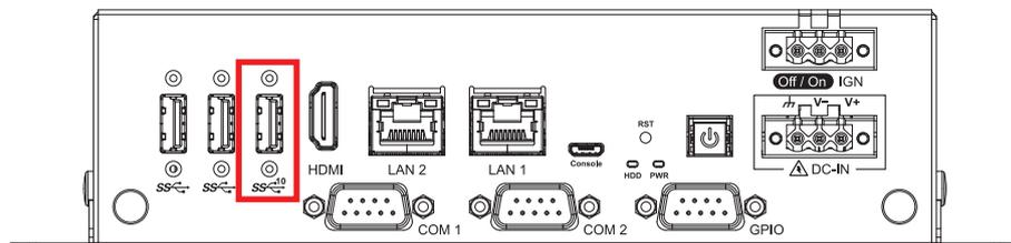
There is a USB 3.2 Connector connections available supporting up to 10Gb per second data rate in the front side of EAC-6000 series. It also compliant with the requirements of Super Speed (SS), high speed (HS), full speed (FS) and low speed (LS).
