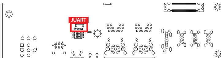
The connector is connected by OOB cable, it can transfer the debug UART signal to OOB, and it will monitor by Ethernet remote the system status. The UART Signal is switched by SW9.
