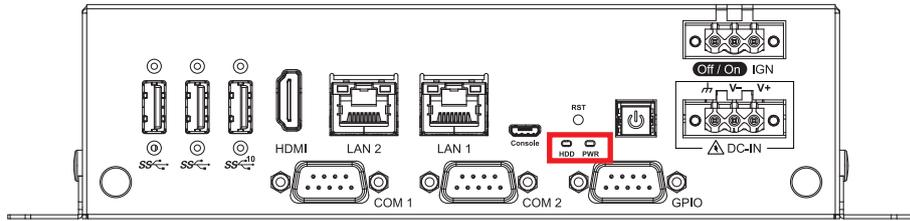
The HDD LED is presented with the storage active status. The PWR LED is presented with power of system is ready.on.normally.
