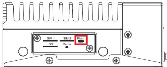
The EAC-6000 USB Recovery mode provides an alternate boot device (USB). In this mode, the system is connected to a host system and boots over USB. This is used when a new image needs to be flashed. USB0 must be available to use as USB Device for USB Recovery Mode.
