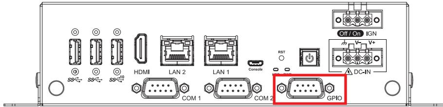
The power voltage of each GPIO pin is 0V to 3.3V. The maximum current can be 20uA.
