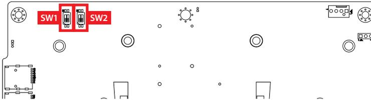
There are two types of Terminal Resistors Internal and External. It can refer below truth table to select resistor type when you want to do.
