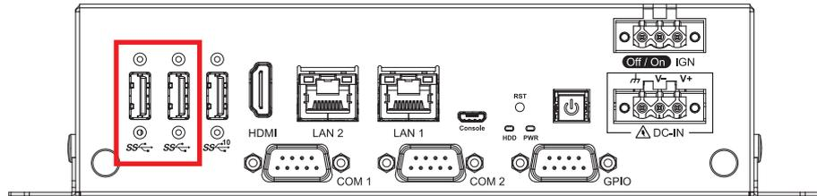
There are 2 USB 3.2 Gen1 Connector connections available supporting up to 5Gb per second data rate in the front panel of EAC-6000 series. It is also compliant with the requirements of Speed (SS), High Speed (HS), Full Speed (FS) and Low Speed (LS).
