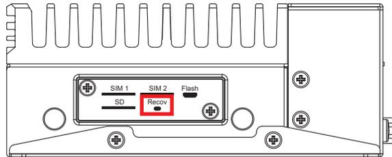
Press the Button enter Force Recovery Mode. Button is held down while either system is first powered on, or by pressing & releasing reset button while Recovery button is pressed.
