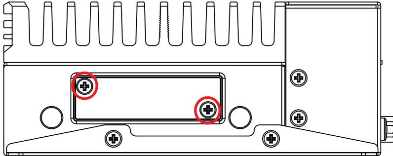
**Step 2** Inserting SD card.
