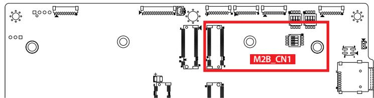
The M.2 key B connector is suitable for applications that use Host I/Fs supported USB 3.0, USB 2.0, it can be plugged including LTE/5G, NvME Module card 3052 type.
