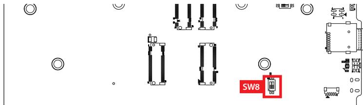
The DIP Switch can change what the function you want for SD card, Audio, UART and OOB function. The SD card and Audio only option 1 can be used. The UART and OOB only option 1. Please refer as below function Table.
