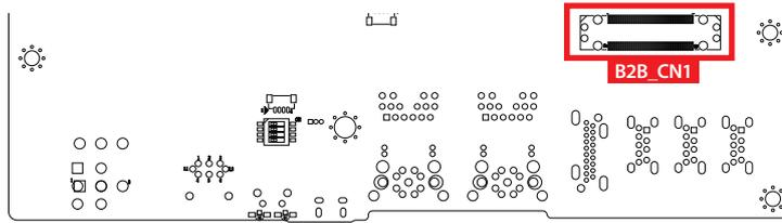
B2B\_CN1 connector apply to EAC-6000-CB and EAC-6000-PE board use. Host I/Fs supported MIPI CSI x4 transfer GMSLx4 with Fakra Connector and PCIe x1 transfer 4 GigE with PoE LAN.
