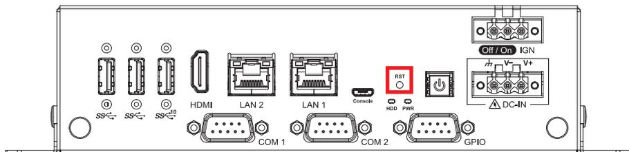
If the system have error or frozen status, you can press Reset Button to restart, then the system will reboot OS.
