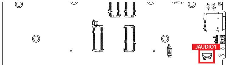
The Connector is connected by Audio Jack Cable for Line-out and Mic In application. It must be switched by DIP SWITCH SW8 (2.4.1.7) if the Audio signal is enabled.
