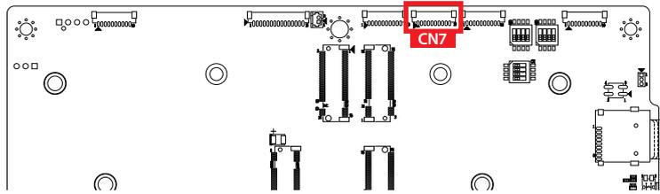
The connector include 7 bit GPIO with 3.3 power level, it can be set GPI or GPO mode what you want.
