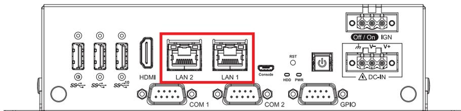
There are two 8-pin RJ-45 jacks supporting 10/100/1000 Mbps Ethernet connections on the front side of EAC-6000 series. It supports 1000BASE-T gigabit data signals over standard Ethernet Cat 5/Cat 6 cable.
