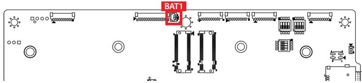
The BAT1 connector is connected by CR2032 with cable supply power for RTC IC, if the battery is disconnected, the RTC function will not be work, and it will have a wrong time of OS.
