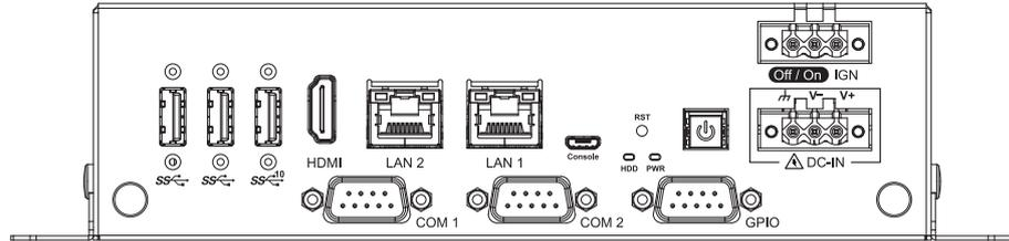
In Vecow EAC-6000 series, Most of the I/O connectors are located on the front panels. Most of the general connections to computer devices, such as POWER CON, IGN CON, COM, USB 3.0, LAN (RJ-45), Digital Display Port, GPIO, POWER BUTTON, RESET BUTTON, LED indicators are placed on the front panel.
