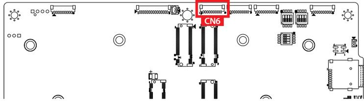
The connector include I2C and SPI bus for reserve application.
