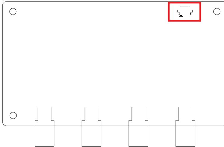
The JMFP Header is connected to the GMSL deserializer FSYNC input.
