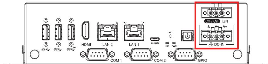
EAC-6000 supports 9V to 50V DC wide range power input by terminal block. It can be divided into Top layer and Bottom layer. The Top layer is Ignition signal control application, and the bottom layer is power source input.
