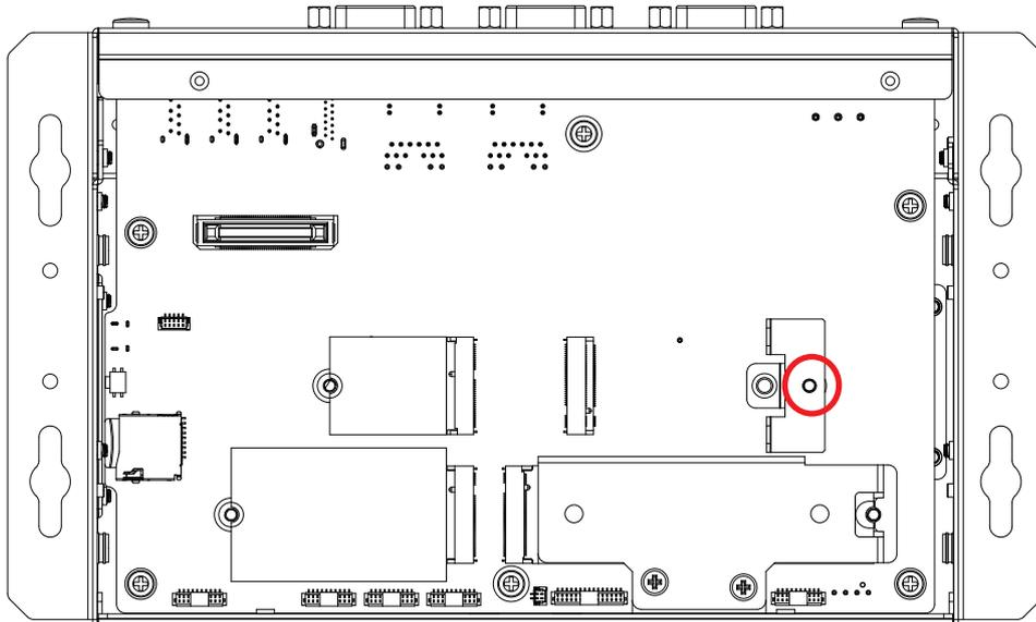
**Step 2** Install M.2 Key B 3042 into slot and fasten one pan head M3x4L screw.
