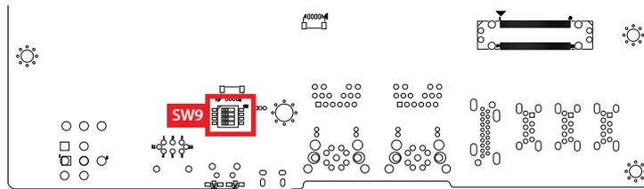
The debug UART is connected to console port (Micro USB), it can monitor what the system status is when the system is booted up. It also can be changed to OOB when use remote control by Ethernet.
