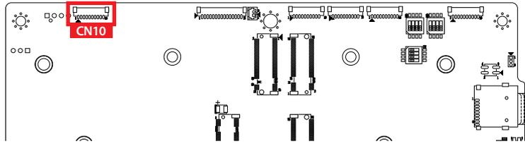
The Connector is suitable for combo applications that use Host I/Fs supported CAN BUS and UART (COM2). It must be switched by DIP SWITCH SW8 (2.4.1.7) if the UART signal is enabled.
