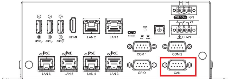
CAN Bus Connector Pin Out:
