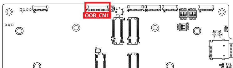
The connector is connected by OOB daughter board, if you want to remote control the system function (Power on / reset or monitor).
