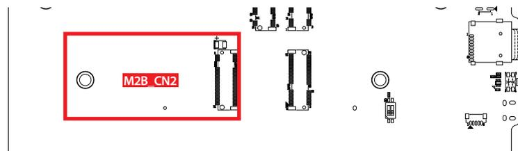
The M.2 key B connector is suitable for applications that use Host I/Fs supported USB 3.0, USB 2.0, it can be plugged including LTE/5G, NvME Module card 3052 type.
