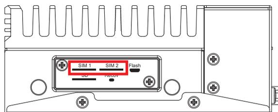
The external Nano SIM card offers wireless communication capability by M.2 key B 4G/5G Card to the system.
