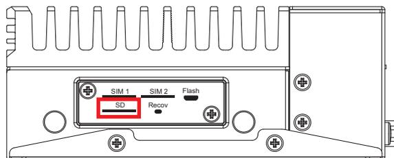
The external Micro SD card provides additional storage expansion. It is located behind the cover-plate on the front panel.
