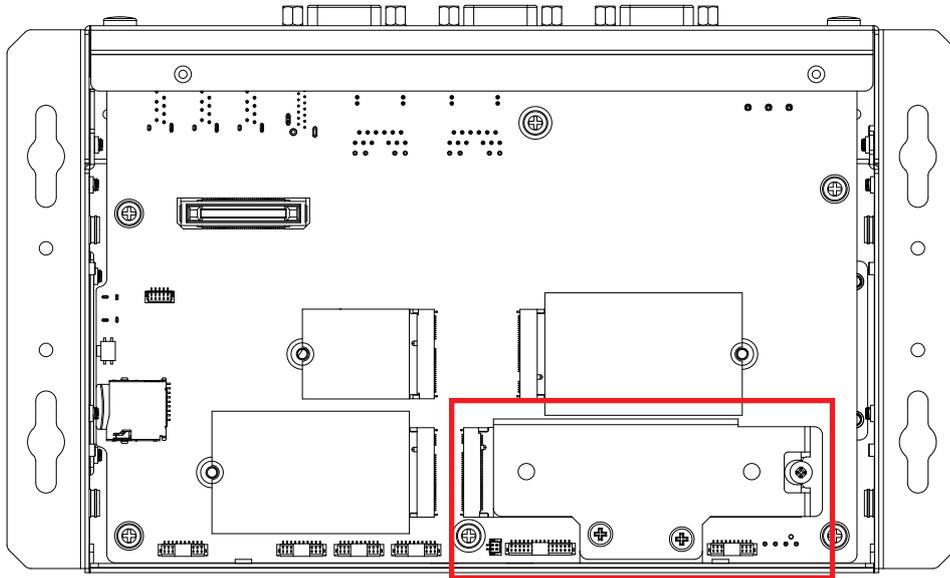
**Step 3** Fasten one pan head M3x4L screw and two F-M3x4L screw.
