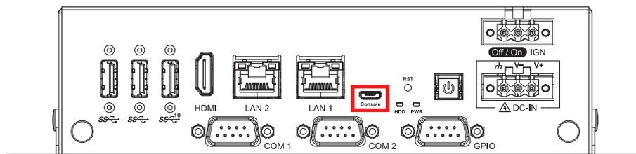
The Console Port is debug Port of system, it connected by Micro USB connector. It can be connected by USB (Type A to Micro USB Type) Cable to USB Port of PC, and execute terminal tool, then it will get the system status message.
