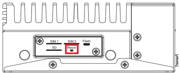
**Step 4:** Keep holding the “Recov” button, and power on the EAC-6000. Continue to hold the “Recov” button at least two seconds, and release.
