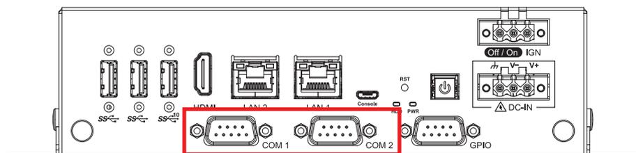
The COM 1,2 can be configured for RS-232, RS-422, or RS-485 with auto flow control communication. The default definition of COM 1 and COM2 is RS-232; if you want to use RS-422 or RS-485, you have to change COM mode the DIP Switch mode select.
