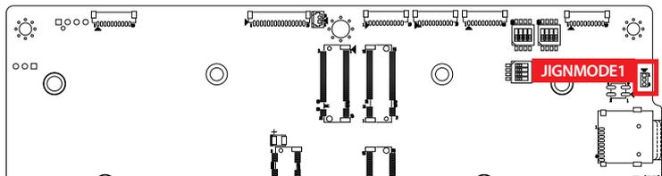
If the system use the ignition mode, the function can be changed by jumper setting. The default is H/W setting, it can be changed by software, but the jumper must be changed Pin 2-3 short.
